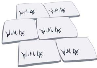
Lay sod in a staggered brick like pattern
