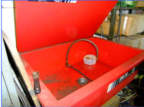
Figure 24: Parts washer in a vehicle maintenance facility. A parts washer should be used to clean parts that have oil or solvents on them. 24
