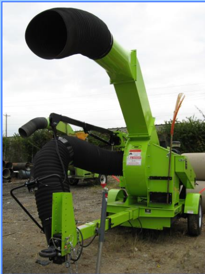
Figure 37: (left) A leaf collector. In the fall, leaves are a source of stormwater pollution because many residents rake their leaves into the street. Leaf collectors will remove leaves which then can be disposed of in a landfill or composted. The important factor in effective leaf pickup is to inform residents in advance to sweep their leaves close to the street, typically the right-of-way, rather than dump them into the street or burn them. 37
