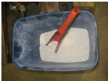
Figure 33: Absorbents. Kitty litter or other absorbents should be used to clean up liquid spills. Any absorbents used to clean up hazardous materials should be treated as hazardous waste and disposed of properly. 33
