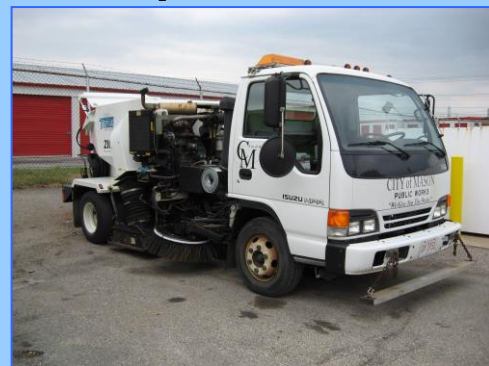
Figure 38: (right) A street sweeper. Street sweeping is necessary to remove dust, dirt, and other pollutants
