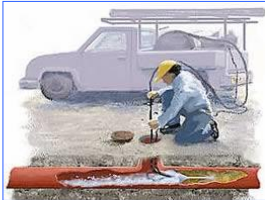
Figure 34: Storm pipe cleaning using the flushing method. Storm drains and pipes should be cleaned at least once a year to remove debris that has collected in the drain. 34
