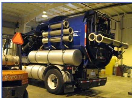
Figure 35: Catch basin vacuum truck. Vacuum trucks pump materials from catch basins to be disposed of in a landfill rather than flushing it into the stream. 35
