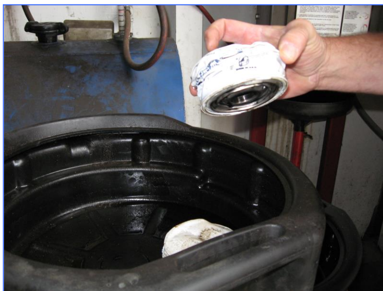
Figure 39: Crushed oil can. Crushing oil cans and recycling oil filters removes excess oil from them and reduces the chance that oil will contaminate streams. 39
