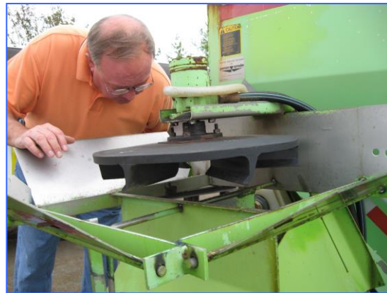
Figure 43: An example of a road salt spreader. Road salt spreaders should be emptied completely when not in use or at the end of the snow season, especially if stored outdoors. Excess salt in spreaders can get washed out in rains. 43
