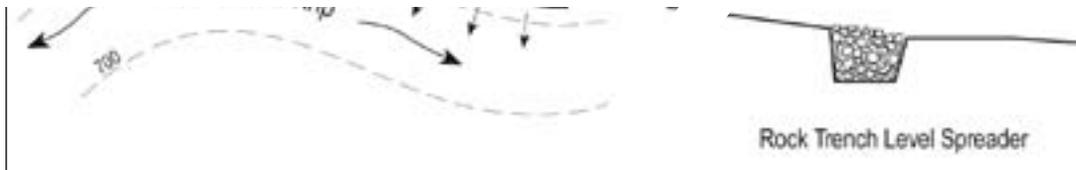
Figure 2.9.2 Grass filter strip with level spreader to direct sheet flow
