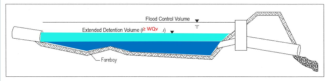
Figure 2.6.5 Wet Storm Water Pond with Extended Detention and Flood Control Volumes
