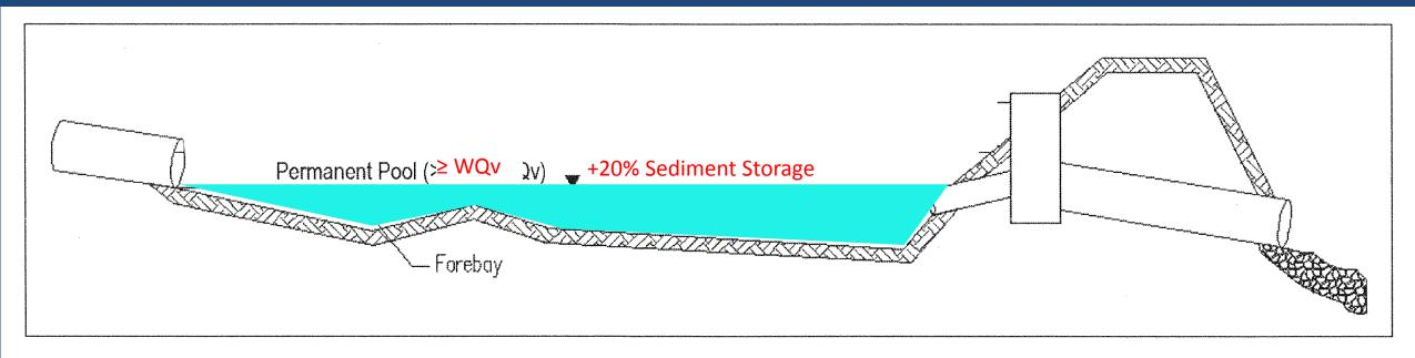
Figure 2.6.5 Wet Storm Water Pond with Extended Detention and Flood Control Volumes
