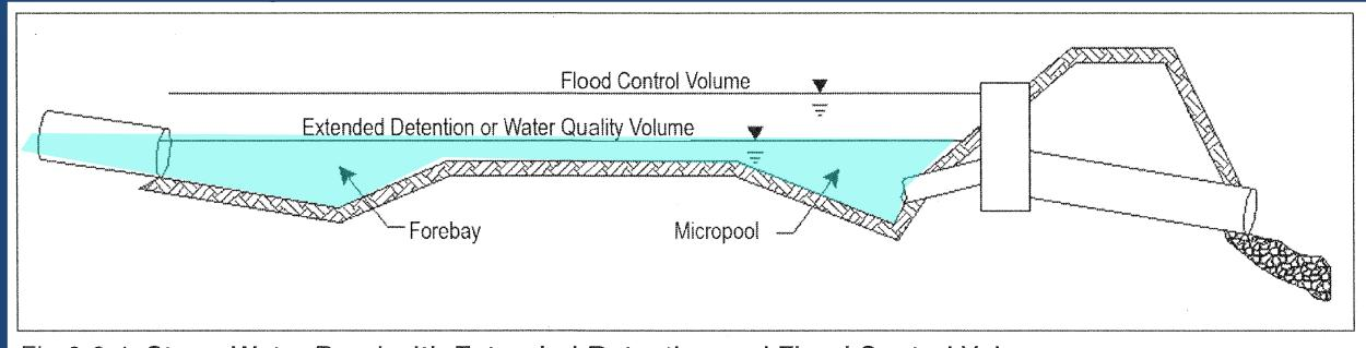
Fig 2.6.4 Storm Water Pond with Extended Detention and Flood Control Volumes
