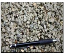
Figure 2.11.6 Pervious Concrete
