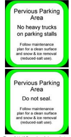
Figure 2.11.13 Examples of signage that might be used to protect pervious pavements.
