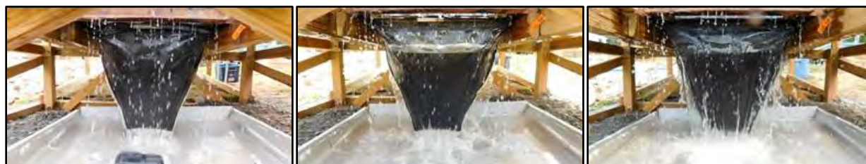
0.06 cfs 0.12 cfs 0.18 cfs (a) FlexStorm® during sheet flow testing with OK110 silica sand.
