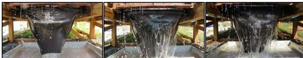
0.06 cfs 0.12 cfs 0.18 cfs (b) FlexStorm® during direct discharge testing with OK110 silica sand
