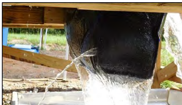
(b) direct discharge with OK110 silica sand
