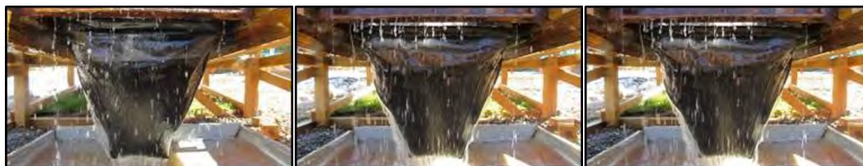
0.06 cfs 0.12 cfs 0.18 cfs (c) FlexStorm® during direct discharge testing with sandy loam soil
